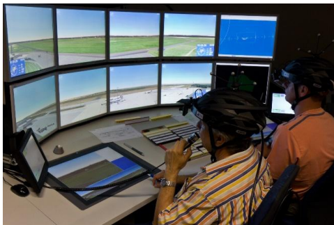
Figure 1: Controllers workplace in Remote Tower Center simulation environment with standard equipment (flight strips, weather display, control zone radar) and video panorama system that replaces out-of-windows view for two remote airports. Microphone for online radio communication with (pseudo) pilots in a separate room driving the simulated air traffic.
